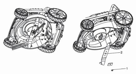
**NOTE:** Be sure to replace the parts in the exact order in which they were removed. When installing the cutting blade, verify that it is installed with the curved ends pointing toward the mower deck, and not toward the ground.
